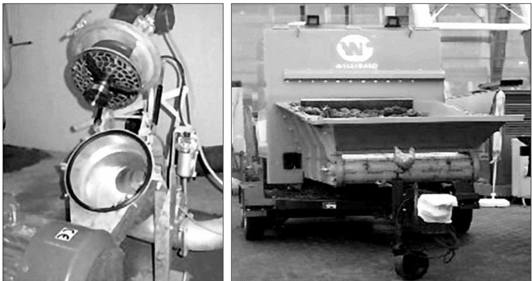
Figure: Perforated disc macerator and external shredder (Photo: Hugo Vogelsang Maschinenbau GmbH, KWS)
